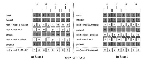
Figure 3.3: ColumnWeaving/S Early Pruning, consisting of the two steps a) step 1, b) step 2, c) connected with bitwise *OR*
