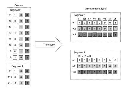
Figure 2.5: Vertical bit parallel method
