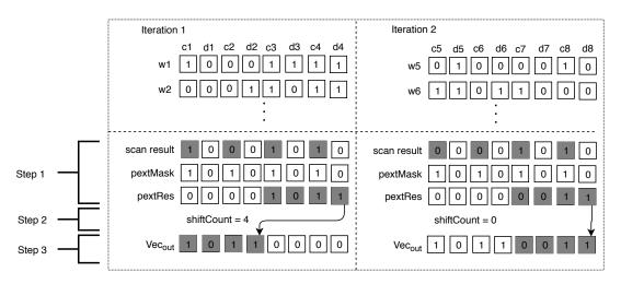
Figure 3.4: ColumnWeaving/S Result Shrink implementation
