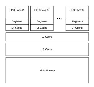
Figure 2.1: Cache hierarchy of modern processors
