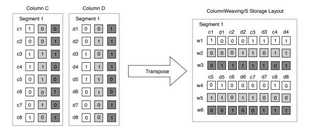
Figure 3.1: ColumnWeaving/S Storage Layout
