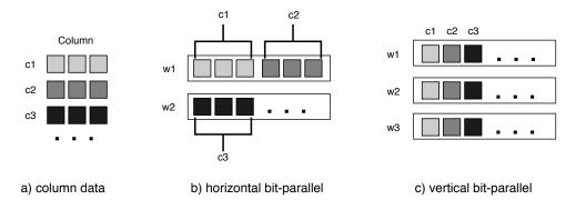
Figure 2.4: a) Sample Column containing 3 3bit codes, b) its encoding using horizontal bit parallel method, c) and vertical bit parallel method
