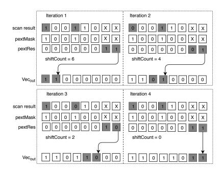
Figure 4.4: ColumnWeaving/L Result Shrink implementation
