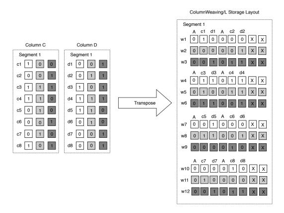
Figure 4.1: ColumnWeaving/L Storage Layout, A additional Bits, X unused bits
