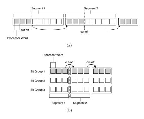
Figure 2.7: Early pruning on a) VBP and b) BitWeaving/V
