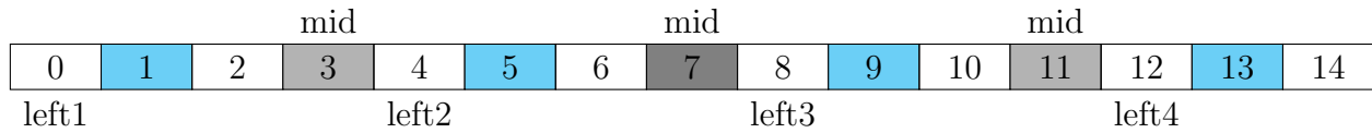
Figure 4.6: Indices used by lowerBoundUniformBinarySearchBranchlessPrefetch4 . The current search range are the keys 0 to 14. 7 is the current separator element, 3 and 11 are the next two possible separator elements. left1 , left2 , left3 and left4 mark the four possible sub-ranges the search can continue with after two search steps. The cache lines holding the keys 1, 5, 9 and 13 are prefetched.
