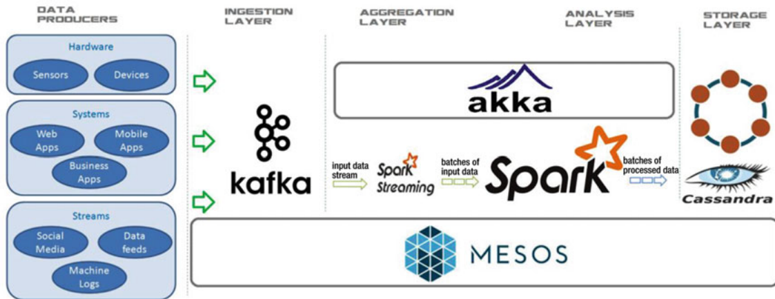
Figure 2.9: SMACK (Apache Spark, Mesos, Akkaa, Cassandra and Kakfa) [ER16a] overview. The graphic shows the roles and connections between each component from the technological stack.
